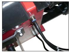
**STEP 10:** Remove the bolt and washer from the Pressing Arm mount located on the front of the Assist Arm Column. Place the Pressing Arm onto the mount and re-install the bolt and washer. Tighten the bolt securely.
