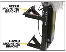
STEP 8: The Assist Arm will attach to the Tire Changer chassis as shown below. Remove the two hex bolts supplied with the machine (arrows). With another person's help, tip the Assist Arm Column upright, so that the brackets line up with the mounting holes. Be careful not to break the plastic air lines. Use the two hex head bolts and washers removed at the beginning of this step, and four matching bolts and washers from the hardware kit. Tighten all six bolts securely with a 16mm wrench.
