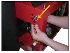
**STEP 5:** Locate the 5-way union located inside the machine. Disconnect the air line indicated by the arrow. Press the short hose on the Hose Tee Assembly into the 5-way air union.
