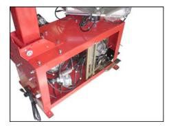
**STEP 3:** If your machine has an Inflator Box Assembly already installed, remove it and set it aside. (This applies to tire changers now in use)
