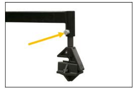
STEP 14: Remove the three Allen head mounting screws at the top of the Assist Arm Column (top left photo) and set them aside. Position the Inflator Box as shown and re-install the screws. Tighten the screws with a 5mm Allen wrench (top right photo). Find the unused 8mm line coming from near the top of the Column, and press it into the fitting on the bottom of the Inflator Box (bottom photo). Re-install the side access cover.
