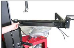
**STEP 12:** Press each of the three marked lines into the matching numbered port on the Assist Arm air control box.
