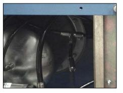
STEP 9: Locate the two loose air lines coming out near the bottom of the Assist Arm Column (arrow). The larger line is 8 mm in diameter. The smaller line is 6 mm in diameter. Press the 8 mm line into the top press lock fitting on the rear of the changer. Press the 6 mm line into the lower fitting.
