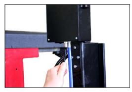
**STEP 15:** Remove the locking pin located on the round tube at the front side of the Assist Arm Column (arrow). Position the Disk Arm as shown and re-install the locking pin. Re-install the machine side cover.
