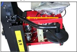
STEP 16: Congratulations! Your Tire Changer Assist Arm is complete. Remember to check all bolts and screws for tightness. Connect air and electrical service to the machine. Set the air regulator between 100 and 116psi, and check thoroughly for air leaks. Test each function and control on the machine as described in the owner's manual BEFORE attempting to change tires. THE TIRE MACHINE SHOULD BE OFF OF THE SKID BEFORE OPERATING.
