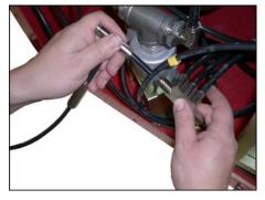
**STEP 6:** Press the line that was disconnected in step 5 into the opposite side of the Hose Tee Assembly's three way air union.
