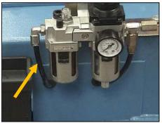
**WARNING:** Do not use the air line connected behind the regulator / filter assembly! This line supplies the bead blast system. Connecting to this line will cause damage to your Assist Arm and its controls. **Be certain** that you are using the correct air line before you continue.
