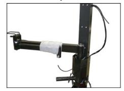
**STEP 11:** Locate the loose air lines coming out near the top of the Assist Arm column. Route the three longest lines (labeled 1, 2, and 3) through the square tube on the back of the Pressing Arm as shown above.
