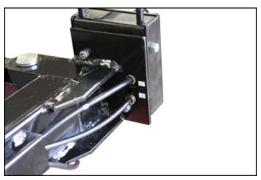
**STEP 13:** Insert the Press Block into the end of the Pressing Arm and tighten the locking bolt with a 16mm wrench. The Press Block must turn freely after the bolt is tightened.
